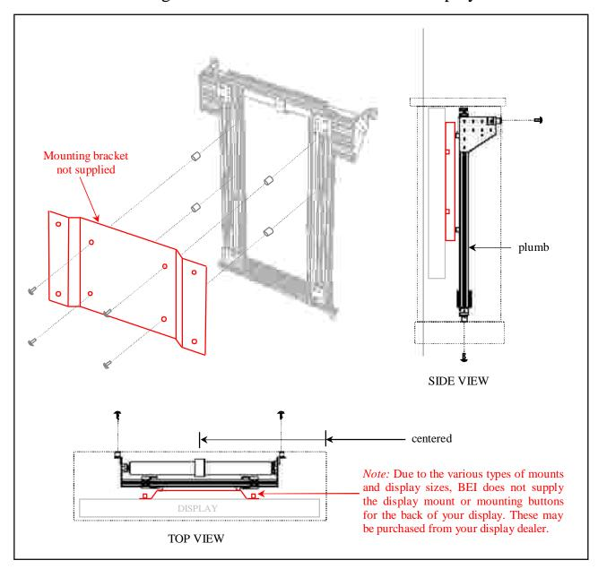
The BEI Motorized Display Lift mounts easily to the inside of any cabinet. The lift is thru-bolted to the cabinet using 4 ea. 5/16-18 x 1-1/4" machine screws with washers into the threaded neoprene shock mounts (BEI supplied this screw length based on a cabinet wall and floor of 5/8" to 3/4". The shock mounts are located at the top back (2 ea.) and the bottom (2 ea.) of the lift frame. When mounting the lift frame, it must be plumb top to bottom and centered side to side within the cabinet.
